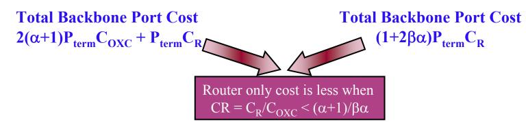
$\begin{aligned} \textbf{C}_{\text{R}} &= \text{router port cost per } \lambda \\ \textbf{C}_{\text{OXC}} &= \textbf{OXC port cost per } \lambda \\ \beta &= \text{factor representing statistical } \\ &= \text{multiplexing} \end{aligned}$
