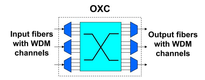
OXC switches signals on input {wavelength<sub>i</sub>, fiber<sub>k</sub>} to output {wavelength<sub>m</sub>, fiber<sub>n</sub>}
