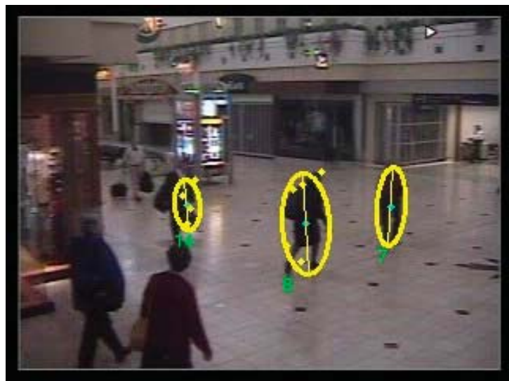
Illustration of automatically measuring the heights of humans as they move across the field of view of a camera. Data courtesy of Honeywell Corporation.
