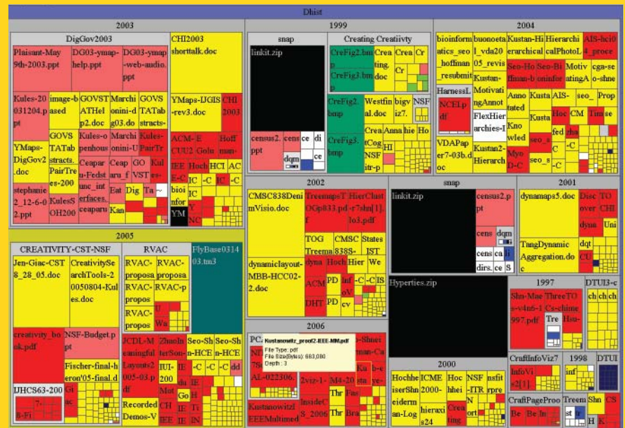
Treemap showing part of a hard drive with folders for recent years, with size of each rectangle proportional to file size in bytes. Color indicates file type, such as red for pdf, light red for ppt, black for zip and yellow for doc. This is a well-organized hierarchy but there is a duplication of two large green bmp files in the 1999 folder.
