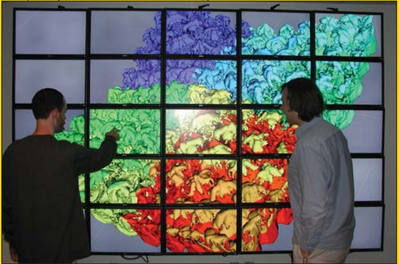
Tiled LCD displays help Varshney and his students look at images in very high resolution. Here, graduate students examine a simulation of how two gases mix.
