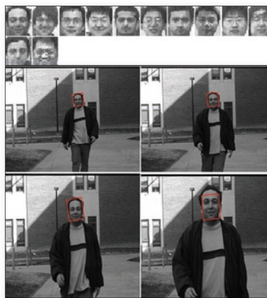
Top: Face gallery images of size 48x42 pixels. Bottom: Sample frame in one probe video. The actual face size ranges from approximately 20x20 in the first frame to 60x60 in the last frame.
