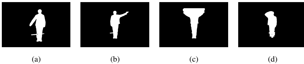
Figure 9: Some of the errors in the background subtraction errors in the control gesture dataset resulting in inaccurate silhouette extraction.
