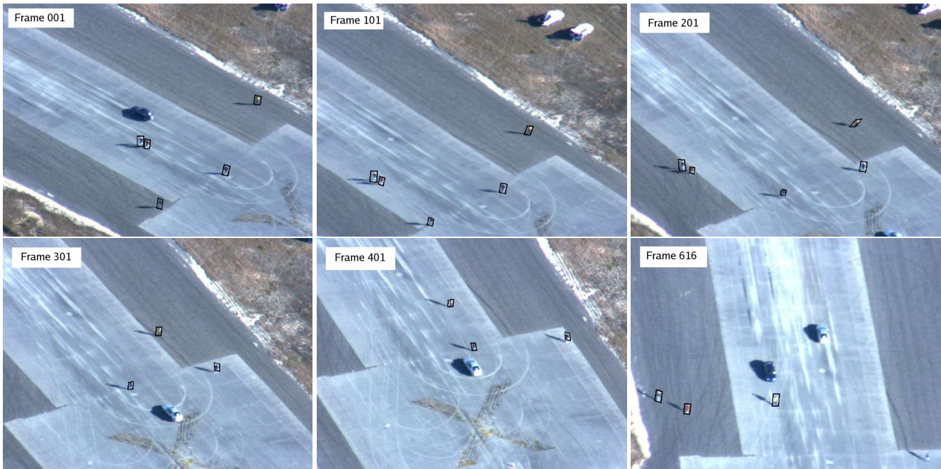
Fig. 2. Tracking multiple targets with a moving camera over 600 frames. Tracking is robust even when targets have less than 10 pixels on them.
