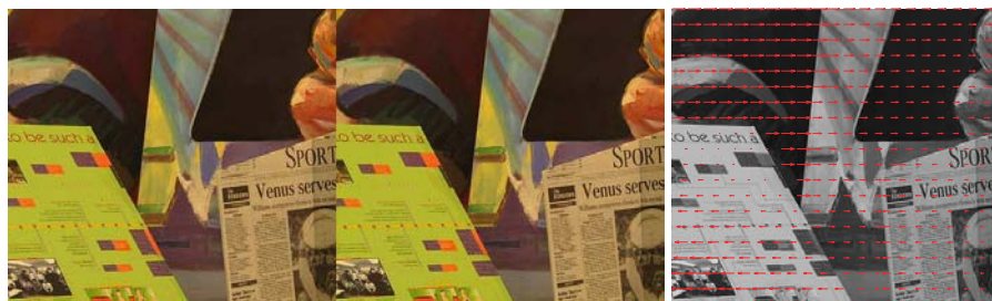
Fig. 2.9 (left) Two images from the Middlebury data set [8], (right) and the optical flow capturing dense motion between the two images.
