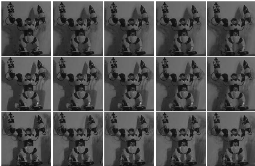
Fig. 7.3 Results of reflectance field acquisition obtained from compressed measurements of various compression factors. Each column corresponds to a different compression factor (L to R: 1.3, 1.7, 2, 2.7, 4), and each row corresponds to a different source direction. Images courtesy [176].
