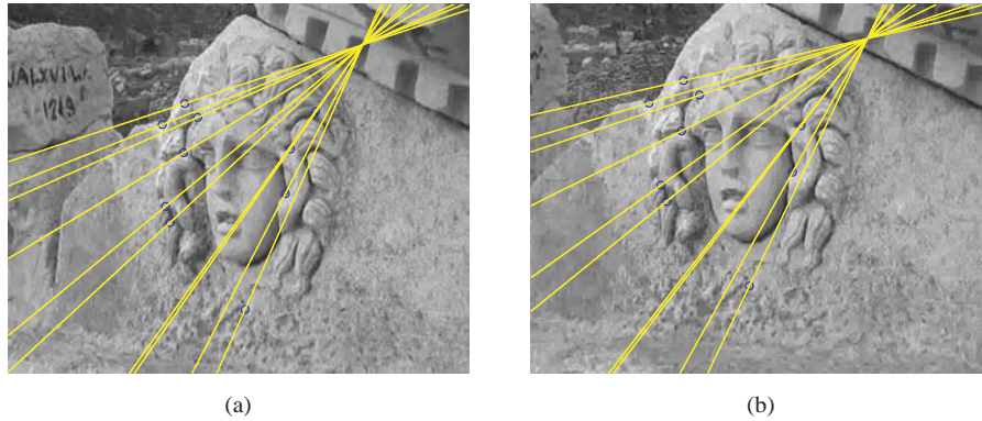
Fig. 2.7 Figure showing two views of a Medusa head. Feature points are shown in small circles. For each feature point and its corresponding point on the other image, we show epipolar lines. The point where the epipolar lines converge is the epipole.
